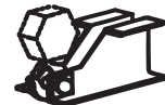
OPTION D Lower Head Room Bails Utilized when headroom must be held to a minimum. Crane hook data must be supplied, see page 56.
