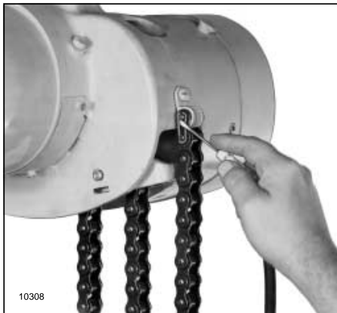
Figure 7-1. Removing Spring Clip from Connecting Link at Tail End of Load Chain (Roller Chain Models)
