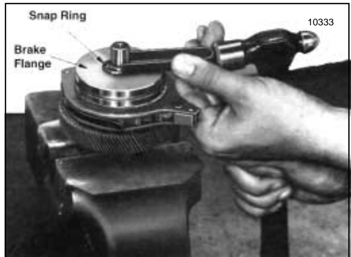
Figure 7-21. Removing Snap Ring from Load Brake Shaft
