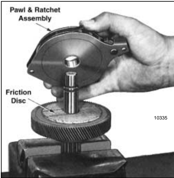
Figure 7-23. Removing Pawl and Ratchet Assembly from Load Brake Shaft
