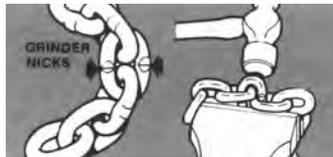
2. Use a 7" (177 mm) minimum diameter by 1/8" (3.1 mm) thick abrasive wheel (or type recommended by wheel supplier) that will clear adjacent links.
