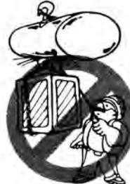
Do not use load chain as a sling. Such usage damages the chain and lower hook.
