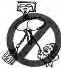
Be sure hoist and load are in a straight line. Do not pull at an angle.
