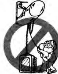
Do not operate with hoist head resting against any object. Lift the load gently. Do not jerk it.
