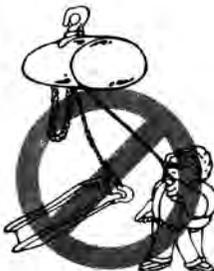
Be sure load is hooked securely. Do not tip load the hook. Do not load hook latch. Hook latch is to prevent detachment of load under slack chain conditions only.
