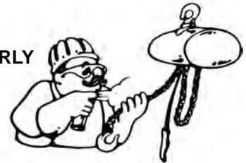
**CLEANING:** Hoists should be kept clean and free of dust, dirt, moisture, etc., which will in any way affect the operation or safety of the equipment.
